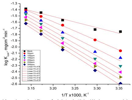
Figure 8: log k (corrosion rate) vs. 1/T curves for Cu in 1 molar Nitric acid in the presence and absence of inconsistent doses of Salazopyrin.
