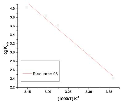
Fig. 10: Log K<sub>ads</sub> vs. (1/T) curves for the corrosion of Cu in one molar Nitric acid in the presence and absence of various doses of Salazopyrin at various temperatures
