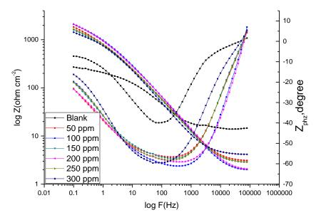
Fig. 4. Bode plot for corrosion of copper in 1 molar Nitric acid without and with various dose of Salazopyrin at 25°C
