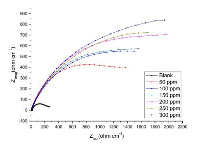
Figure 3. Nyquist plots showing effect of increments concentration of Salazopyrin on corrosion of copper in 1 molar Nitric acid
