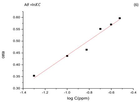
Figure 7: Temkin isotherm curve for Cu in one molar Nitric acid with inconsistent doses of Salazopyrin at 25°C
