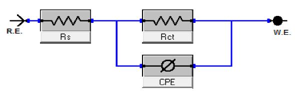
Figure 5. Equivalent circuit model utilized to fit the spectra of impedance
