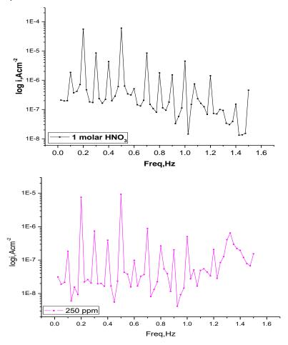
Figure 6: EFM plots for the Cu corrosion in one molar Nitric acid with 250 ppm and without doses of Salazopyrin at 25°C
