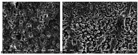
Figure 11: SEM figure of copper surface (a) before putting in 1 molar Nitric acid, (b) after 24 h of immersion in 1 molar Nitric acid, (C-G) after one day of putting in 1 molar Nitric acid +300 ppm of Salazopyrin at 25°C in different magnification power.
