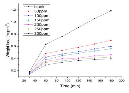
Figure 1: time -mass reduction diagrams for the corrosion of Cu in 1 Molar Nitric acid in the presence and absence of different doses of Salazopyrin at 25°C
