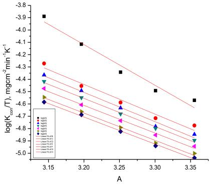
Figure 9: 1/T vs. log k /T plots for Cu in one Molar Nitric acid in the presence and absence of inconsistent doses of Salazopyrin.
