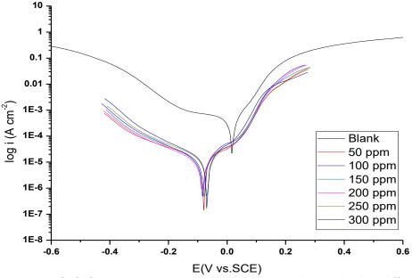
Figure 2: diagram of tafel for the copper corrosion in one molar Nitric acid with and without different dose of Salazopyrin at room temperature.
